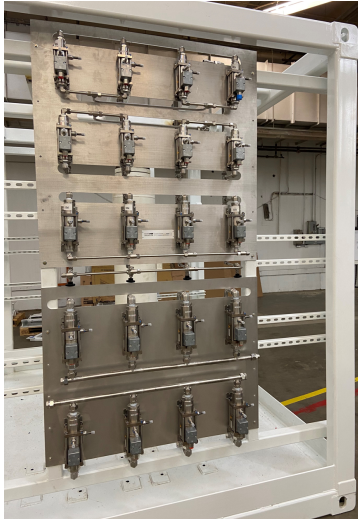
coax® valves integrated into a flow control system
