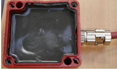
Figure 5-1-2: Terminal box with soldered connection cable
