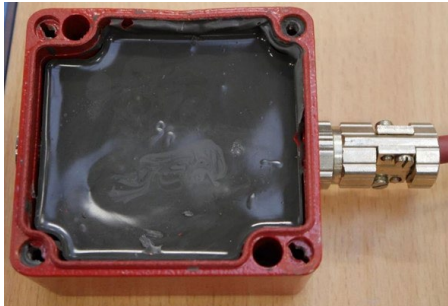
Figure 5 3-2: Terminal box with soldered connection cable
