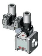
**picture1: Valve deactivatet (open/low pressure mode).** Voltage on pilot valves off and pressure regulators are not actuated.
