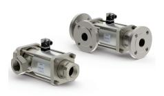
3/2 way valve direct acting pressure range PN 0-16 bar orifice DN 40 mm connection thread/flange
