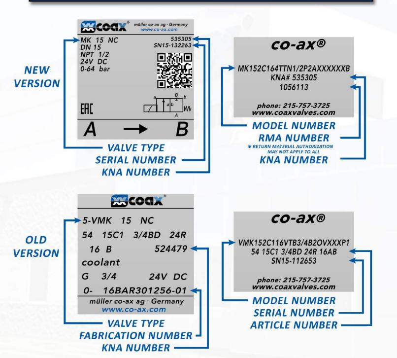
The sample labels above are pointing out the location of the required information that is needed in order to provide the exact specification of a particular valve.
